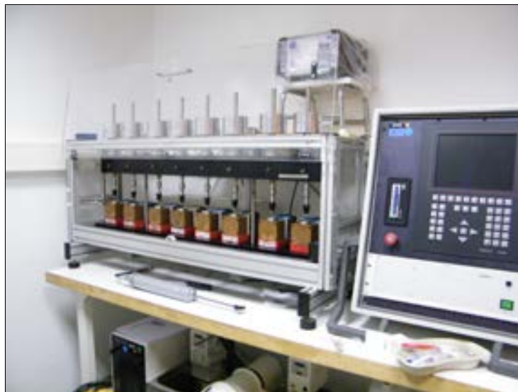
Fig. 2: Assembled test devices in the chewing simulator .
