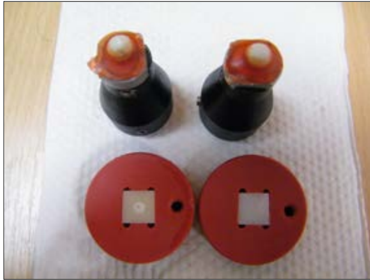
Fig. 3: Embedded Steatite balls in the antagonist holder (top), and samples after finishing the wear test (left: Ceramco®3, right: BruxZir; sample No. 10 each).
